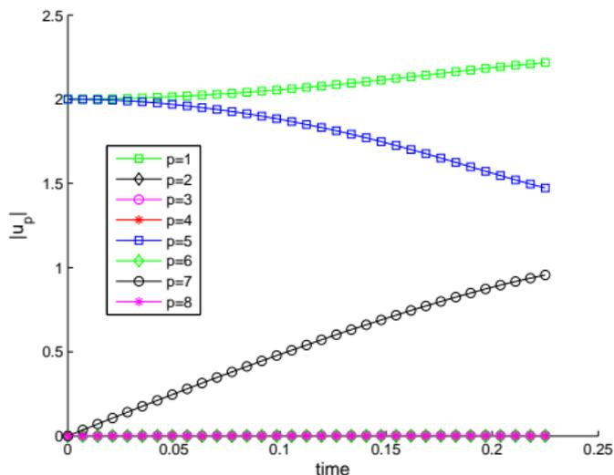
**Figure:** Evolution of modes 1 to 8 in the cubic NLS: modes 1 and 5 feed mode 7 (and only this mode).
